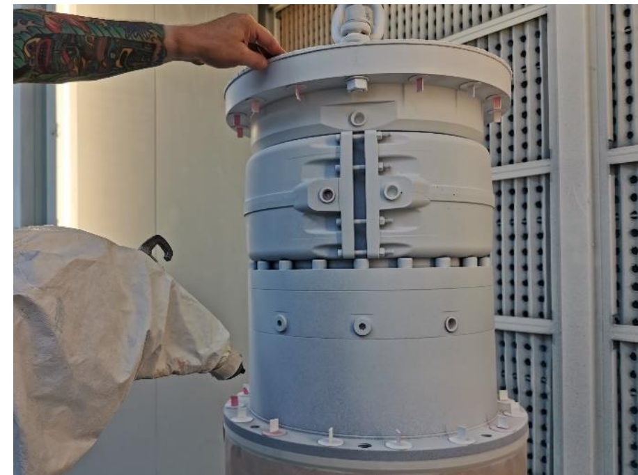
Painting of the refurbished unit
