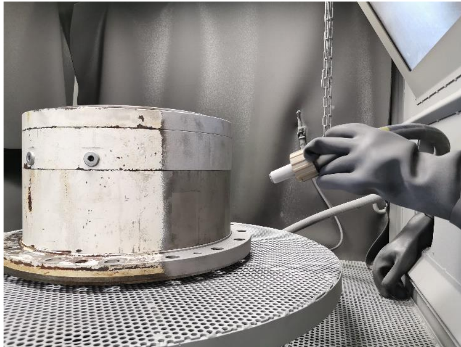
Conservative sand blasting for removal of painting
